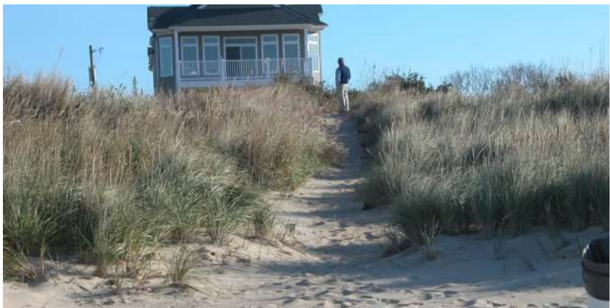
Figure 9. Example of an effective access path through dunes where no dune walkover is needed.
